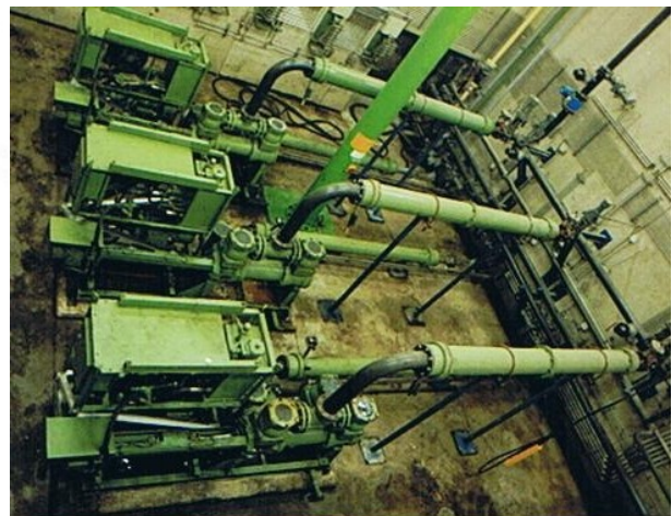
pipe dampener in suction and discharge line of KH-Pumps
